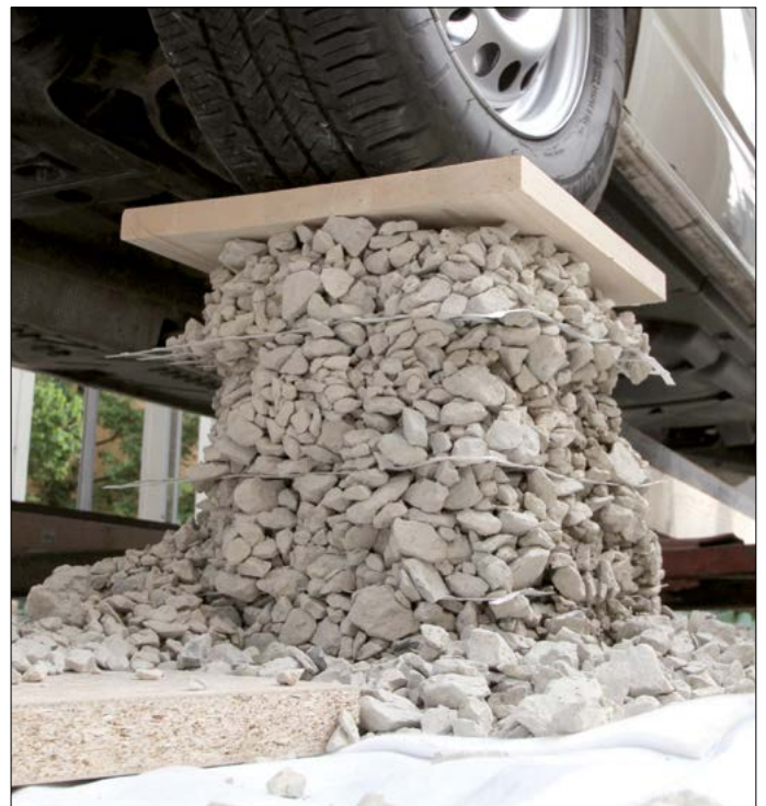
Fig. 10 Demonstration of the interlock effect with a car standing on a Secugrid® reinforced gravel column
