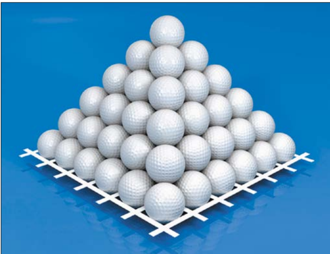
Fig. 9 Naue Secugrid® works because of an interlocking with the soil aggregate (here schematic demonstrated with golf balls)
