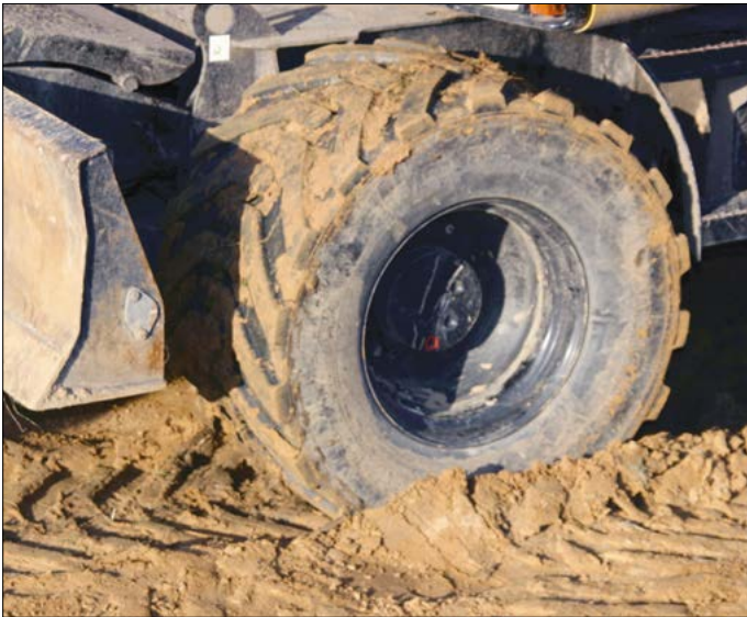
Fig. 16 Truck tire creating rutting on weak subsoil
